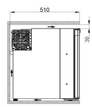
The second method of installation is ventilated through the ventilation grille behind the refrigerator, and the ventilation hole is necessary. The Minimum hole size of the recess is W383mm×D510mm×H535mm.
